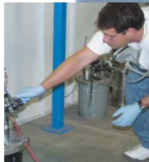
Brian Gedlinske makes a fluid pressure adjustment during a demonstration on pressure-feed airspray equipment.
