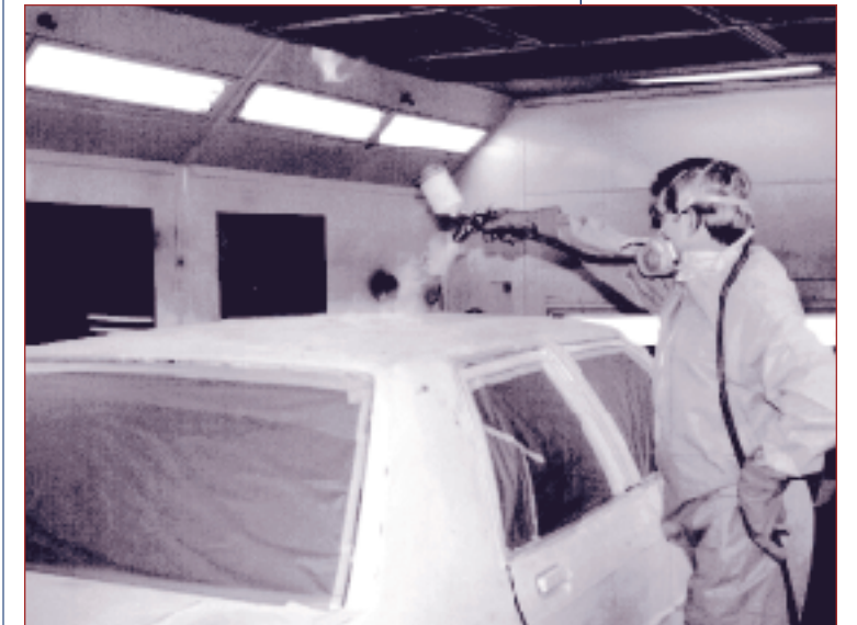
Figure 17: Application of the Primer-Sealer
