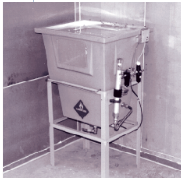
Figure 12: Enclosed Air Powered Mechanical Cleaning System
